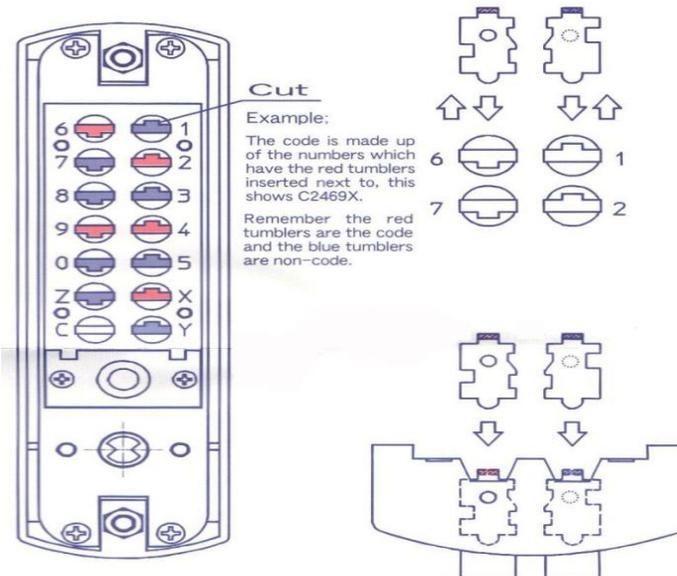
Using the tumblers provided, the code can be changed from a 3 digit to a 7 digit number, always prefixed by C to clear. To increase the numbers in the combination, remove the **blue** and add the red tumblers. To decrease the numbers in the combination, remove the red tumblers and add the blue. (If you insert a tumbler in the wrong position, press the C button and lift the tumbler out.) Now that combination has been changed, release the C button.
