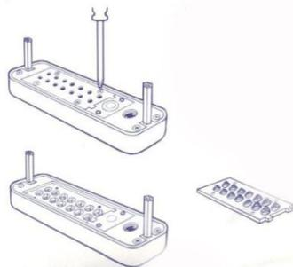
Failure to follow the instructions could result in damage to your lock so please read carefully. Hold the outside body in the horizontal position. Remove the 4 red screws. Carefully remove the plate, as there are many springs attached to it.
